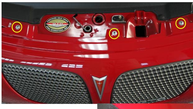
these front tabs is to push on the bumper towards the rear of the car while, as gently as possible, pulling the bumper cover off the brackets. I was successful in removing the bumper without breaking anything.
